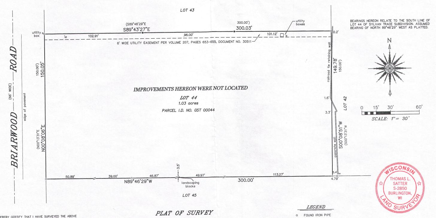
"I HEREBY CERTIFY THAT I HAVE SURVEYED THE ABOVE DESCRIBED PROPERTY AND THAT THE ABOVE MAP IS A CORRECT REPRESENTATION THEREOF AND SHOWS THE SIZE AND LOCATION OF THE PROPERTY, ITS EXTERIOR BOUNDARIES, BOUNDARY FENCES, APPARENT EASEMENTS, ROADWAYS AND ENCROACHMENTS, IF ANY."
